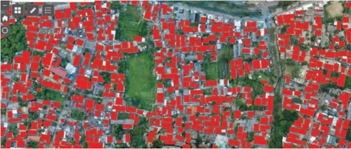
Building footprint counting and extraction
